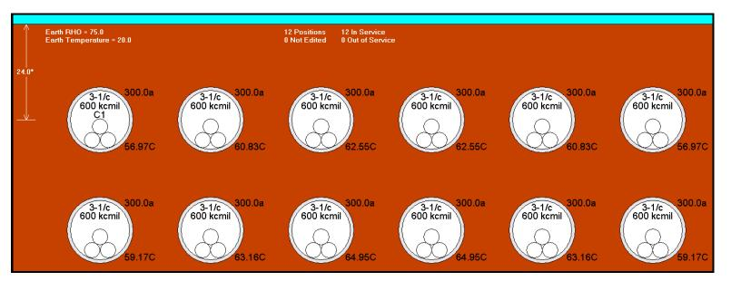
Additionally, these programs will calculate the total loss of energy due to heating and the voltage drop of the conductor. The energy wasted through the conductors due to heat loss can be a significant number and should be considered with any evaluation of these type of electrical duct banks.
