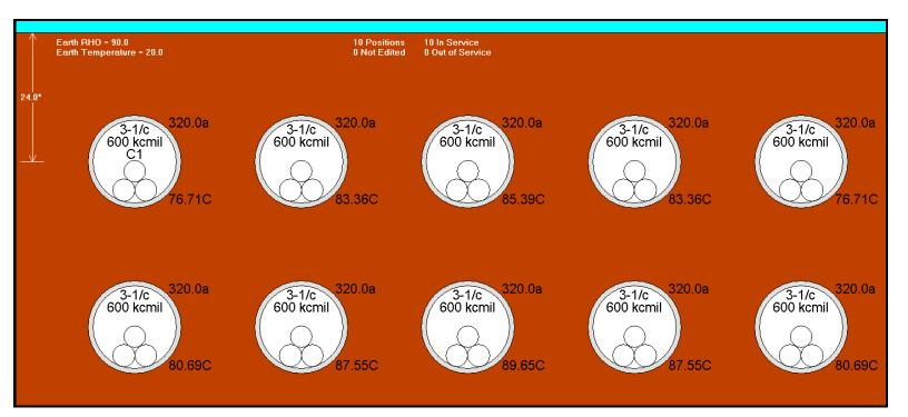
Many data center installation may require de rating, these heating calculations may be critical to ensure that the designed electrical duct bank is adequate to serve the anticipated loads based on the assumed load factor, RHO factor and duct bank configurations.
